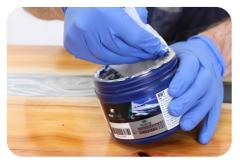
When polishing GlassCast® 50 it is extremely important that all sanding and flatting with the sander and abrasive papers has been done properly. If you find that when you start polishing the resin you can see swirls or scratches emerging in the surface of the resin, this indicates that the sanding and flatting has not been done correctly and the sanding process will need to be repeated.
