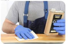
Your choice of wood finish is a matter of personal taste as different products will provide different levels of protection and varying finished appearances. It is also important to seal and finish the wood before we do the final polish of the GlassCast® river. By sealing the wood first it helps avoid the wood being marked by the polishing process; we used a clear Danish Oil.
