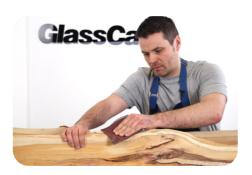
Then use some 80 grit abrasive paper to rub back any loose material left on the de-barked edge to ensure the edge is left as smooth as possible ready for the next stage.
