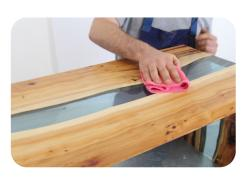
Liberally apply your chosen polishing compound to the satin finished resin and then use a power polisher with a medium to hard polishing pad to polish the surface. Keep topping up the NW1 as needed until it reaches full gloss.
